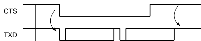
Figure 34-29. Transmitter Behavior when Operating with Hardware Handshaking
