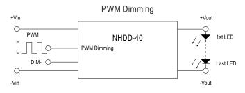
H: >1.5~5VDC or open circuit L: <0.9VDC or short
