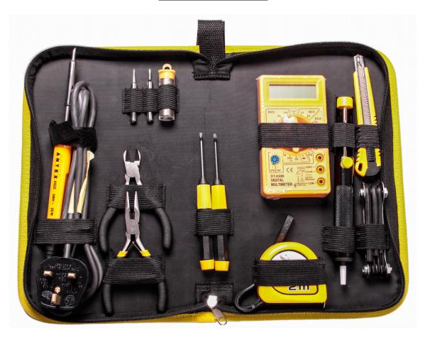
An engineers toolkit featuring an Antex XS25 burn-proof silicone cabled iron, a variety of tools, and a digital multimeter. The tip fitted to the iron is a long life, iron plated Antex 50 bit (2.3mm). Iron power is 25 watts. CE approved.
