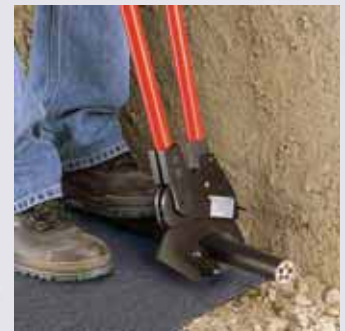
95 31 870: Large cutting capacity: maximum 100 mm dia. / 960 mm 2
