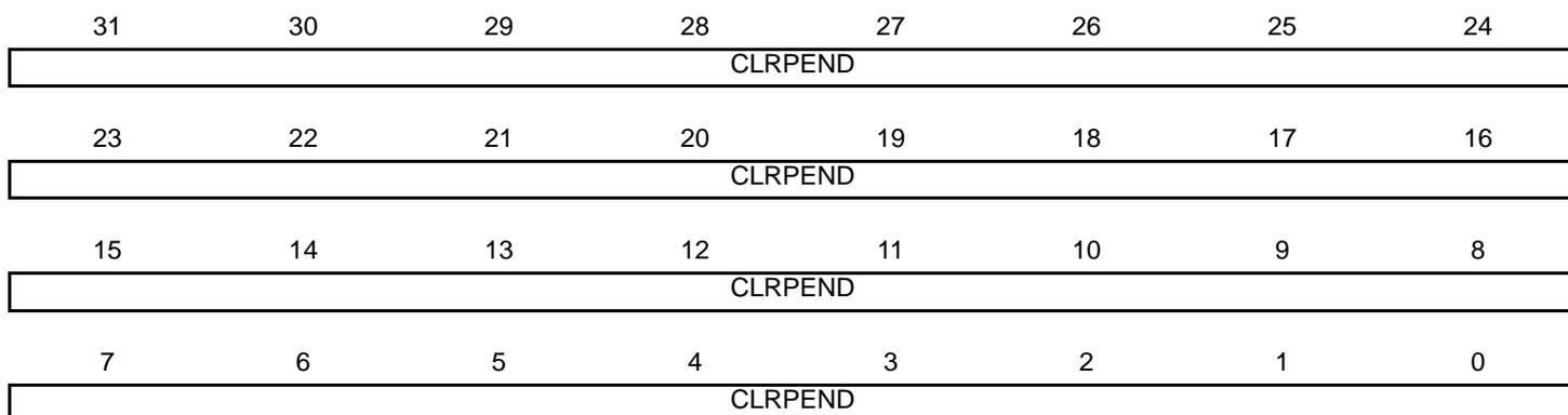
These registers remove the pending state from interrupts, and show which interrupts are pending.
