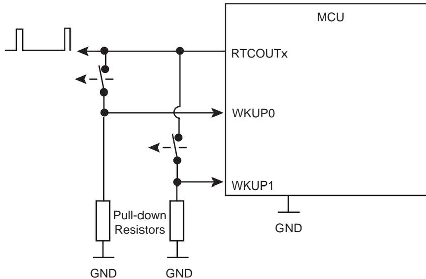
The debouncing period duration is configurable. The period is made for all debouncers (i.e., the duration cannot be adjusted separately for each debouncer). The number of successive identical samples to wake up the system can be configured from 2 up to 8 in the LPDBC field of SUPC\_WUMR. The period of time between two samples can be configured by programming the TPERIOD field in the RTC\_MR. Power parameters can be adjusted by modifying the period of time in the THIGH field in RTC\_MR.
