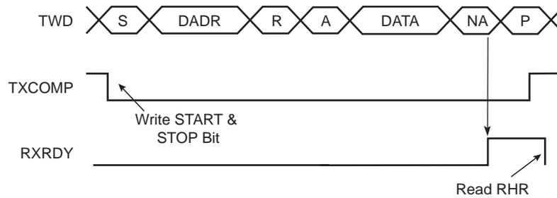
**Figure 36-10. Master Read with Multiple Data Bytes**
