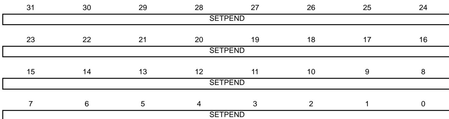
These registers force interrupts into the pending state, and show which interrupts are pending.
