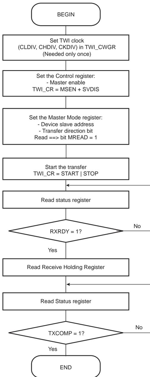
Figure 36-20. TWI Read Operation with Single Data Byte and Internal Address
