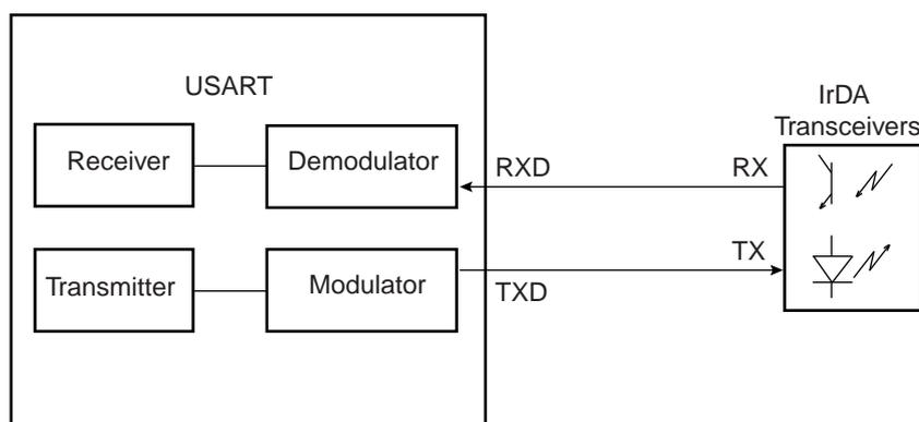
The receiver and the transmitter must be enabled or disabled depending on the direction of the transmission to be managed.
