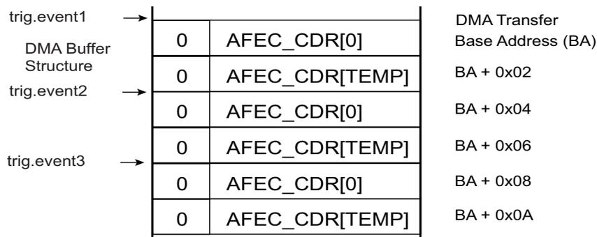
The temperature factor having a slow variation rate and potentially being totally different from the other conversion channels, the AFE Controller allows a different way of triggering the measure when RTCT bit is set in the AFEC\_TEMPMPR but the CH15 is cleared in the AFEC\_CHSR.
