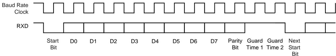
**Figure 38-32. T = 0 Protocol with Parity Error**
