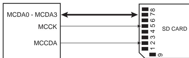
Note: When several HSMCI (x HSMCI) are embedded in a product, MCCK refers to HSMCIx\_CK, MCCDA to HSMCIx\_CDA, MCDy to HSMCIx\_DAy.
