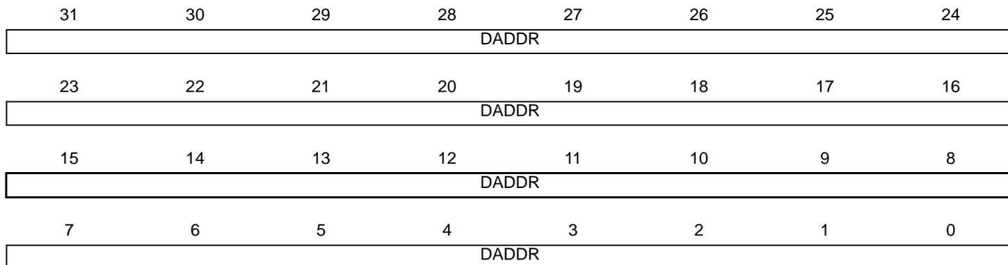
This register can only be written if the WPEN bit is cleared in [“DMAC Write Protect Mode Register”](#).
