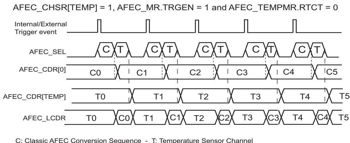
Assuming AFEC\_CHSR[0] = 1 and AFEC\_CHSR[TEMP] = 1 where TEMP is the index of the temperature sensor channel
