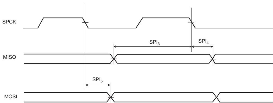
**Figure 47-21. SPI Slave Mode with (CPOL=0 and NCPHA=1) or (CPOL=1 and NCPHA=0)**
