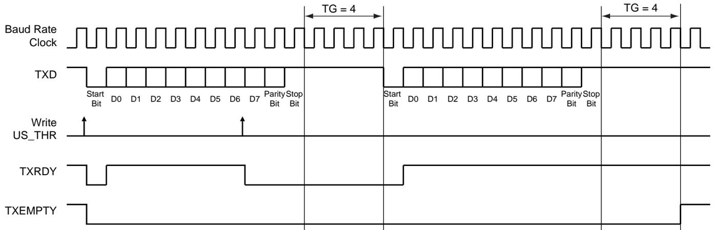
Table 38-10 indicates the maximum length of a timeguard period that the transmitter can handle in relation to the function of the baud rate.
