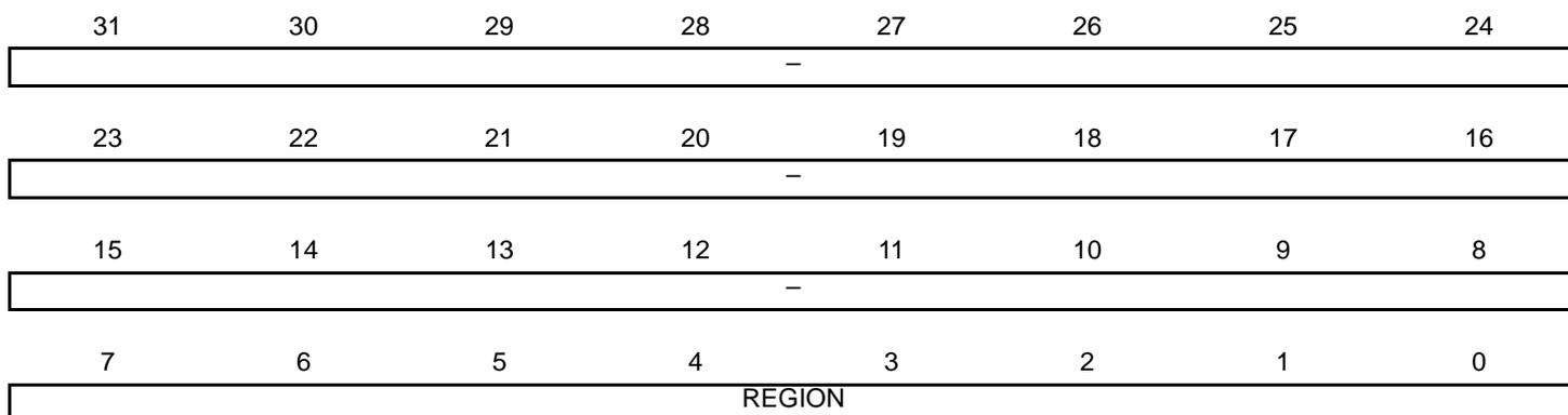
The MPU\_RNR selects which memory region is referenced by the MPU\_RBAR and MPU\_RASRs.
