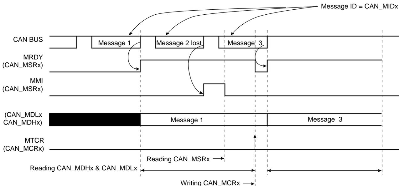
Note: In the case of ARM architecture, CAN\_MSRx, CAN\_MDLx, CAN\_MDHx can be read using an optimized ldm assembler instruction.
