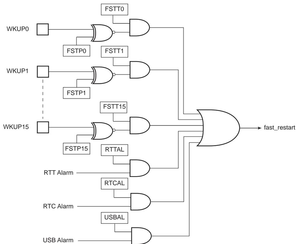
Each wake-up input pin and alarm can be enabled to generate a fast startup event by setting the corresponding bit in PMC\_FSMR.
