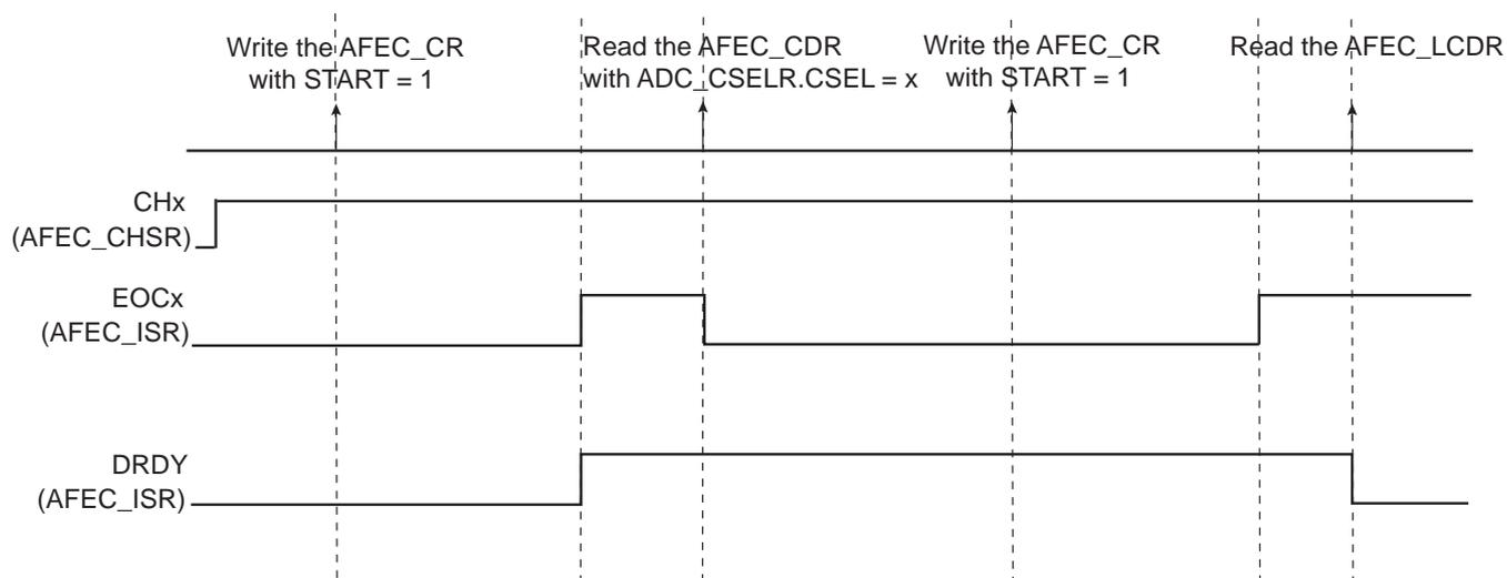
If the AFEC\_CDR is not read before further incoming data is converted, the corresponding Overrun Error (OVREx) flag is set in the Overrun Status Register (AFEC\_OVER).
