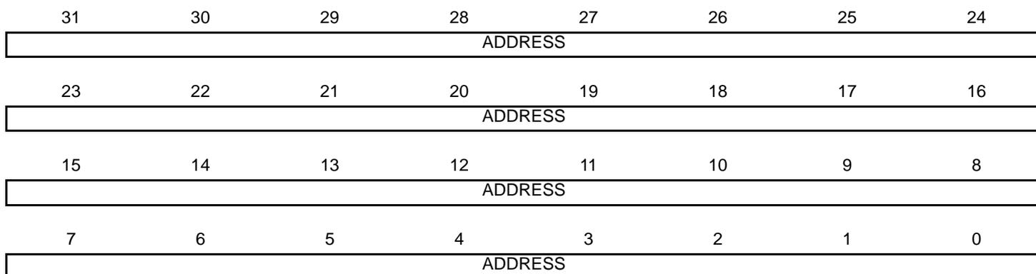
The SCB\_BFAR contains the address of the location that generated a bus fault.
