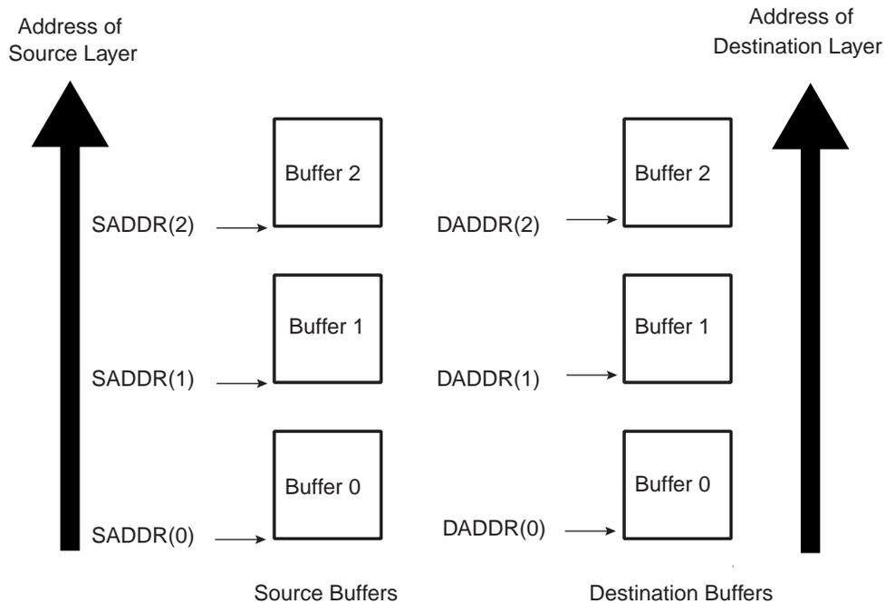
If the user needs to execute a DMAC transfer where the source and destination address are contiguous but the amount of data to be transferred is greater than the maximum buffer size DMAC\_CTRLAx.BTSIZE, then this can be achieved using the type of multi-buffer transfer as shown in [Figure 26-6 on page 477](#).
