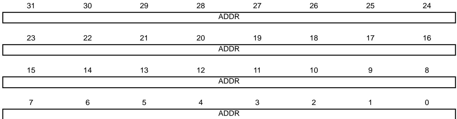
The addresses stored in the Specific Address Registers are deactivated at reset or when their corresponding Specific Address Register Bottom is written. They are activated when Specific Address Register Top is written.
