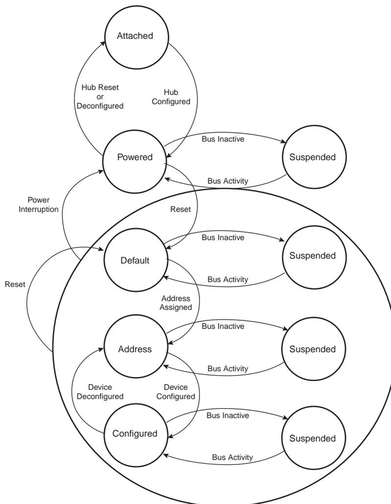
Movement from one state to another depends on the USB bus state or on standard requests sent through control transactions via the default endpoint (endpoint 0).
