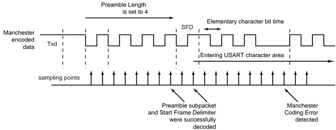
When the start frame delimiter is a sync pattern (ONEBIT field to 0), both command and data delimiter are supported. If a valid sync is detected, the received character is written as RXCHR field in the US\_RHR register and the RXSYNH is updated. RXCHR is set to 1 when the received character is a command, and it is set to 0 if the received character is a data. This mechanism alleviates and simplifies the direct memory access as the character contains its own sync field in the same register.
