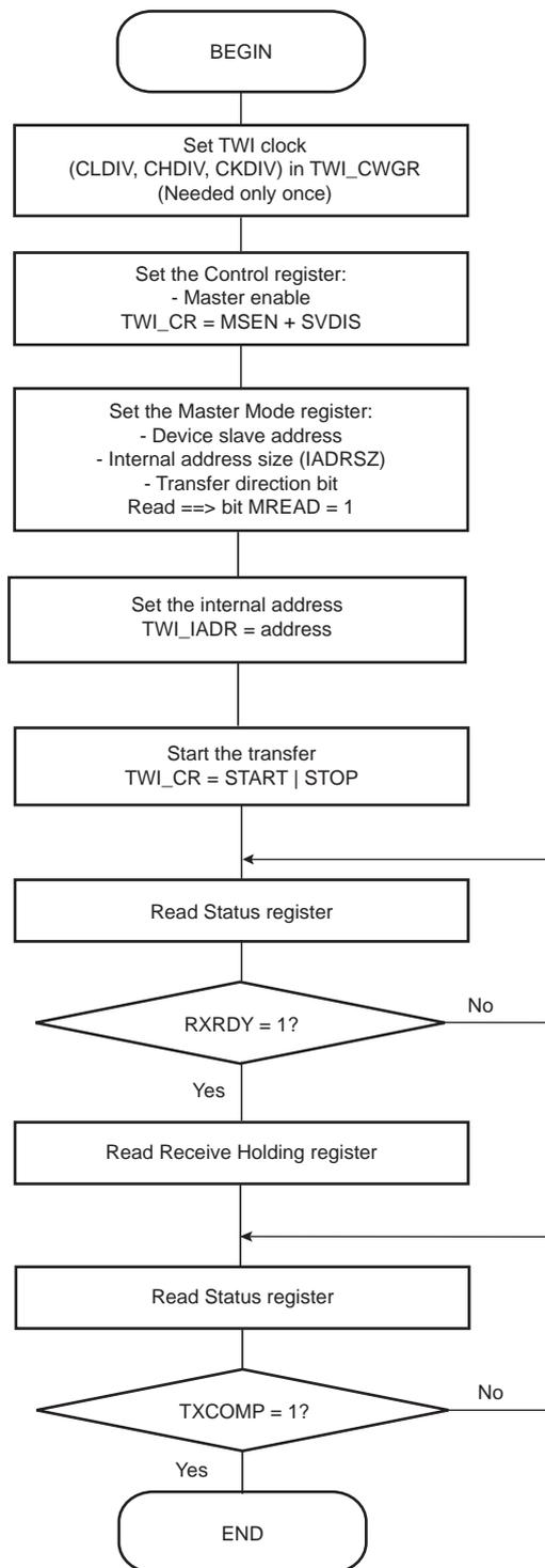
Figure 36-21. TWI Read Operation with Multiple Data Bytes with or without Internal Address
