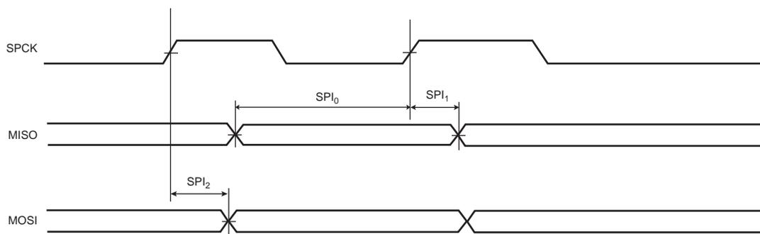
**Figure 47-20. SPI Master Mode with (CPOL = 0 and NCPHA=1) or (CPOL=1 and NCPHA= 0)**
