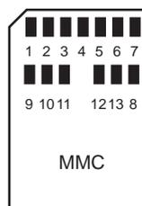
The High Speed MultiMedia Card communication is based on a 13-pin serial bus interface. It has three communication lines and four supply lines.
