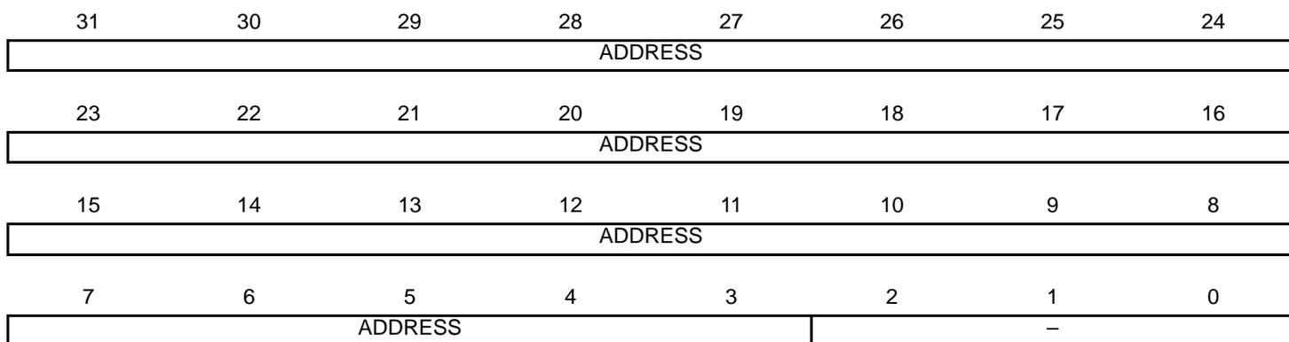
The FPCAR holds the location of the unpopulated floating-point register space allocated on an exception stack frame.
