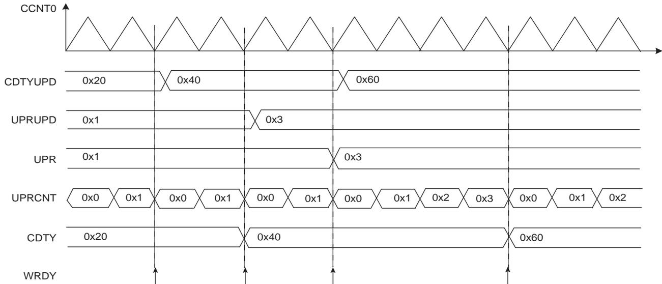
*Method 3: Automatic write of duty-cycle values and automatic trigger of the update*
