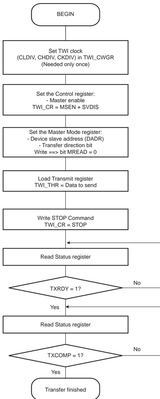
Figure 36-17. TWI Write Operation with Single Data Byte and Internal Address
