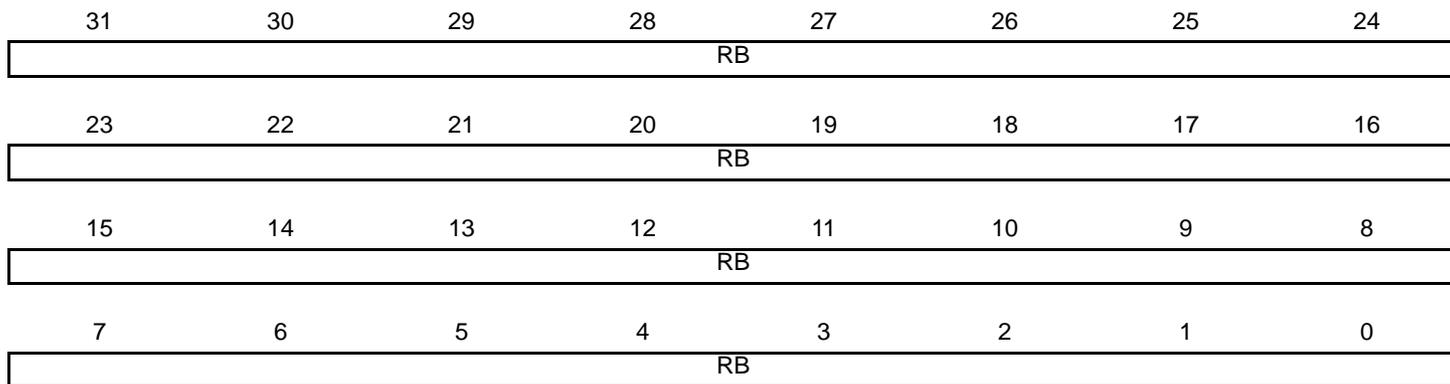
This register can only be written if the WPEN bit is cleared in the [TC Write Protection Mode Register](#).
