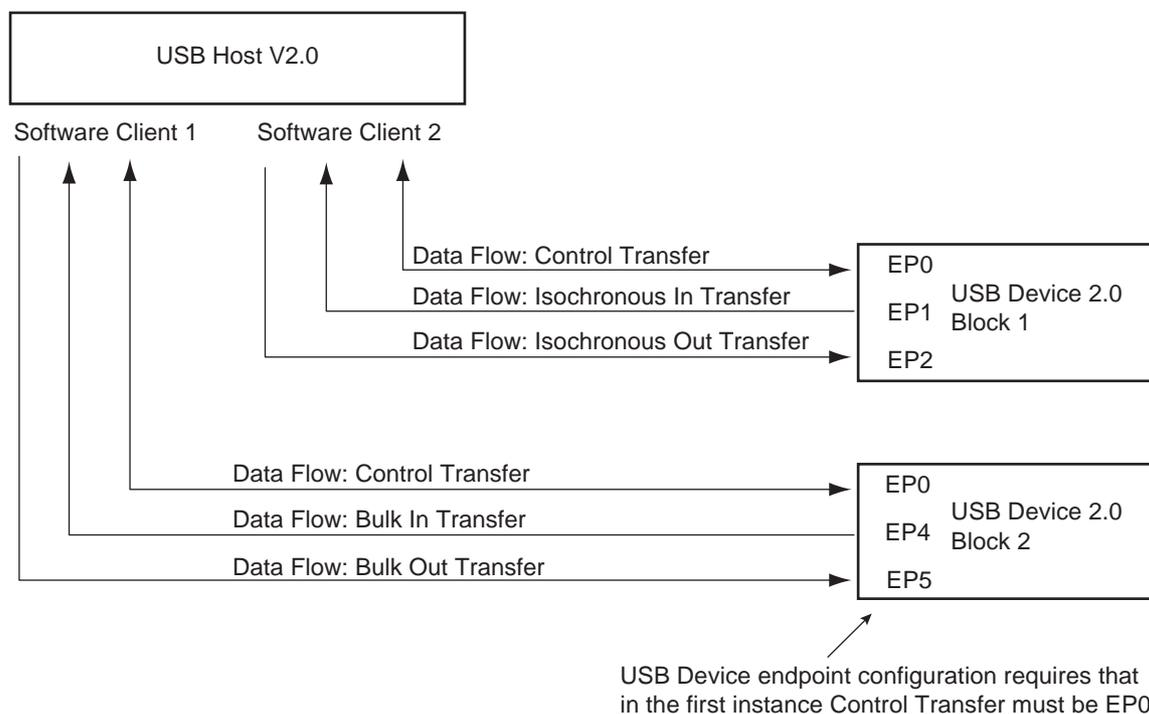
The Control Transfer endpoint EP0 is always used when a USB device is first configured (USB 2.0 specifications).
