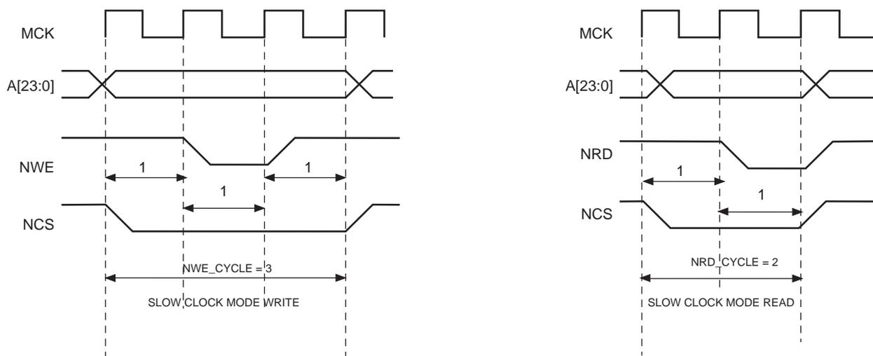
Table 28-4. Read and Write Timing Parameters in Slow Clock Mode
