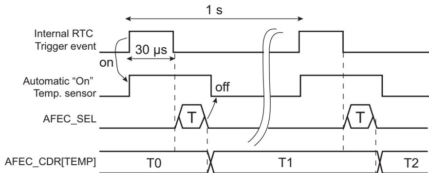
Moreover, it is possible to raise a flag only if there is predefined change in the temperature measure. The user can define a range of temperature or a threshold in the AFEC\_TEMPCWR and the mode of comparison that can be
