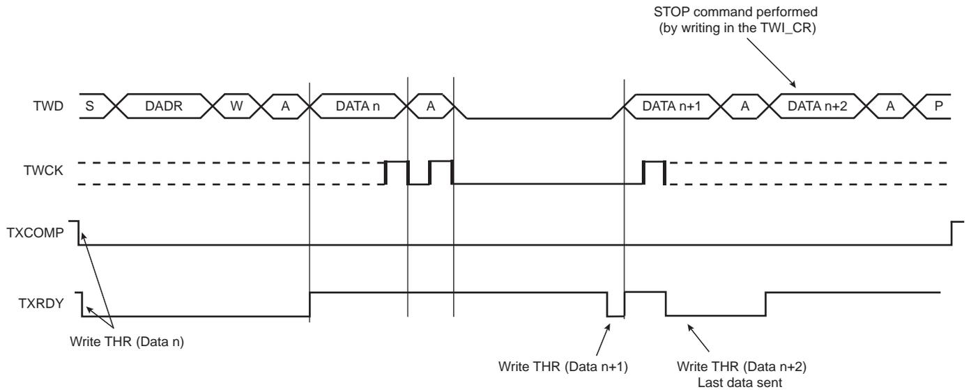
**Figure 36-8. Master Write with One Byte Internal Address and Multiple Data Bytes**
