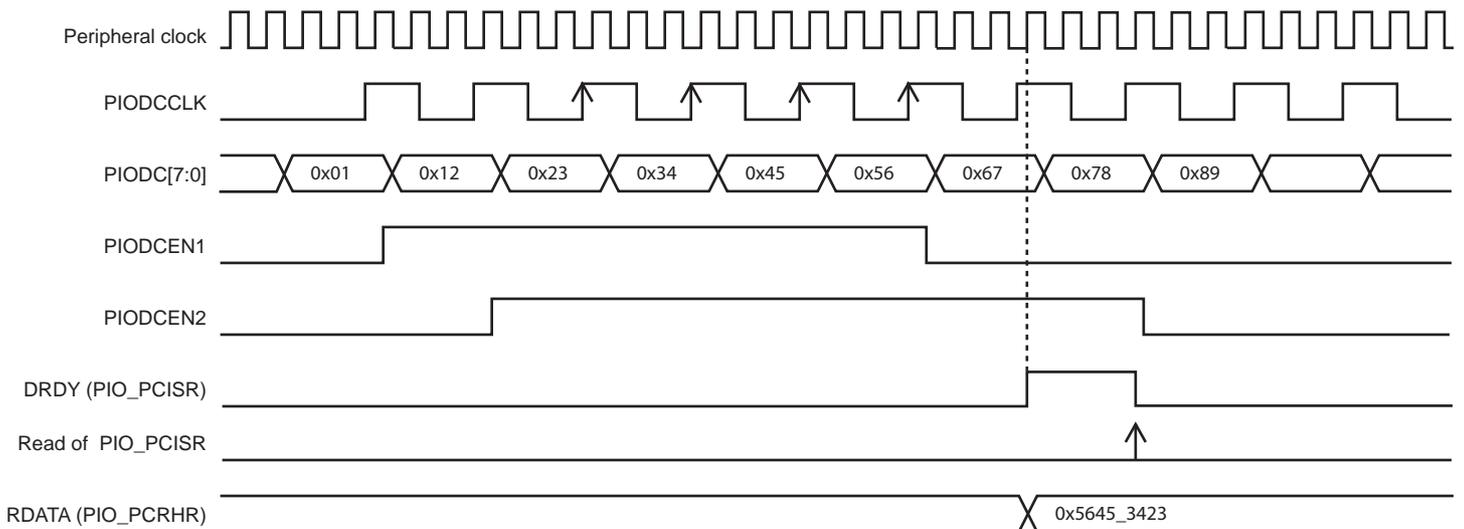
**Figure 34-12. Parallel Capture Mode Waveforms (DSIZE = 2, ALWAYS = 1, HALFS = 0)**
