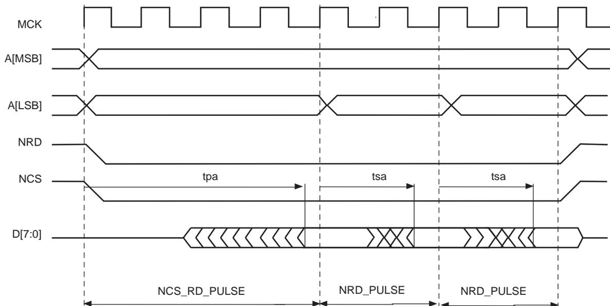
The NRD and NCS signals are held low during all read transfers, whatever the programmed values of the setup and hold timings in the User Interface may be. Moreover, the NRD and NCS timings are identical. The pulse length of the first access to the page is defined with the NCS\_RD\_PULSE field of the SMC\_PULSE register. The pulse length of subsequent accesses within the page are defined using the NRD\_PULSE parameter.
