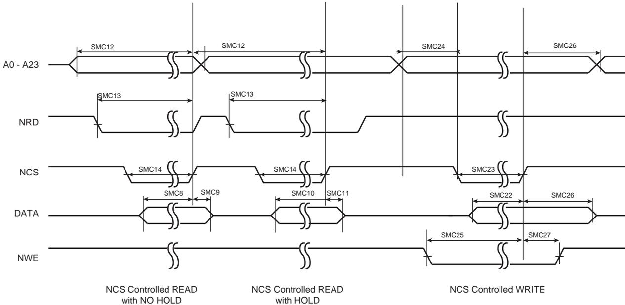
**Figure 47-24. SMC Timings - NRD Controlled Read and NWE Controlled Write**
