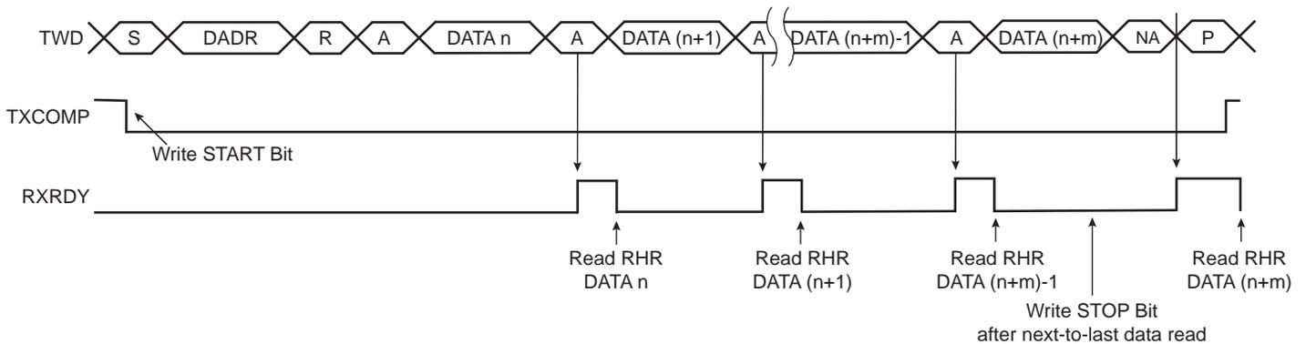
**Figure 36-11. Master Read Clock Stretching with Multiple Data Bytes**
