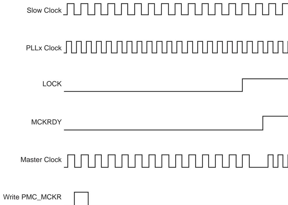
**Figure 30-7. Switch Master Clock from Main Clock to Slow Clock**
