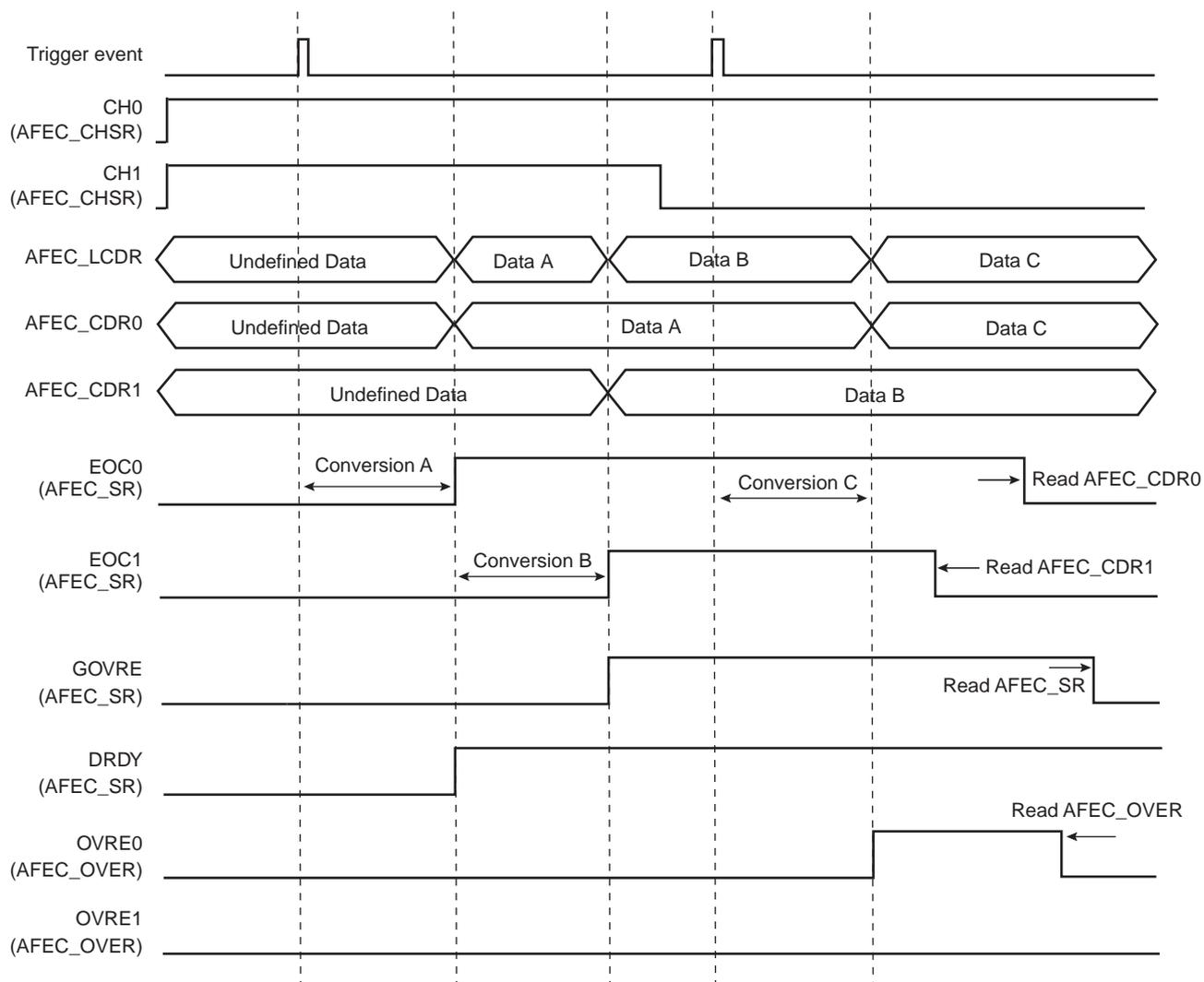
**Warning:** If the corresponding channel is disabled during a conversion or if it is disabled and then reenabled during a conversion, its associated data and its corresponding EOC and OVRE flags in AFEC\_SR are unpredictable.
