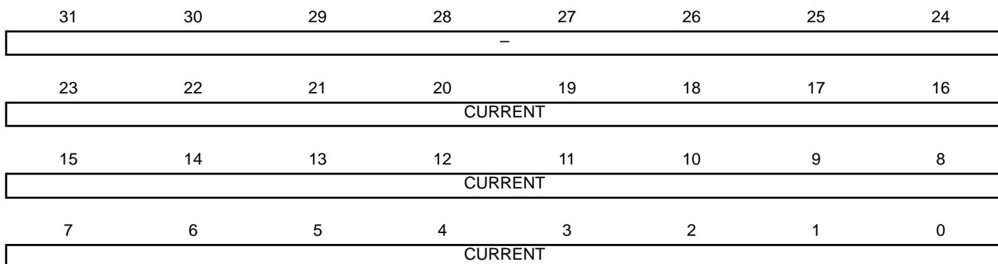
The SysTick SYST\_CVR contains the current value of the SysTick counter.
