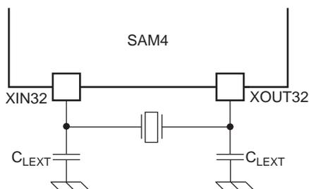
$$C_{LEXT} = 2 \times (C_{CRYSTAL} - C_{PARA} - C_{PCB})$$
