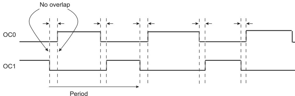
Note: 1. See [Figure 40-5 on page 1027](#) for a detailed description of center-aligned waveforms.
