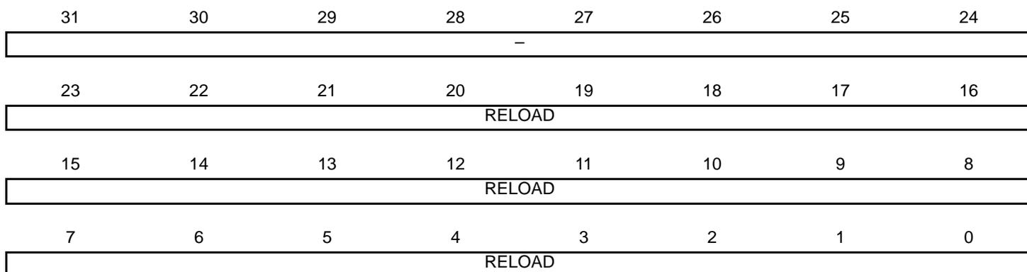
The SYST\_RVR specifies the start value to load into the SYST\_CVR.
