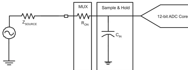
During the tracking phase, the ADC needs to track the input signal during the tracking time shown below:
