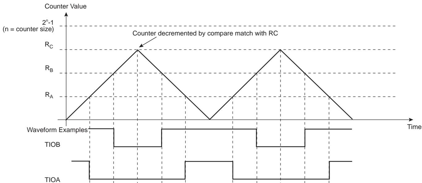
**Figure 39-15. WAVSEL = 11 with Trigger**
