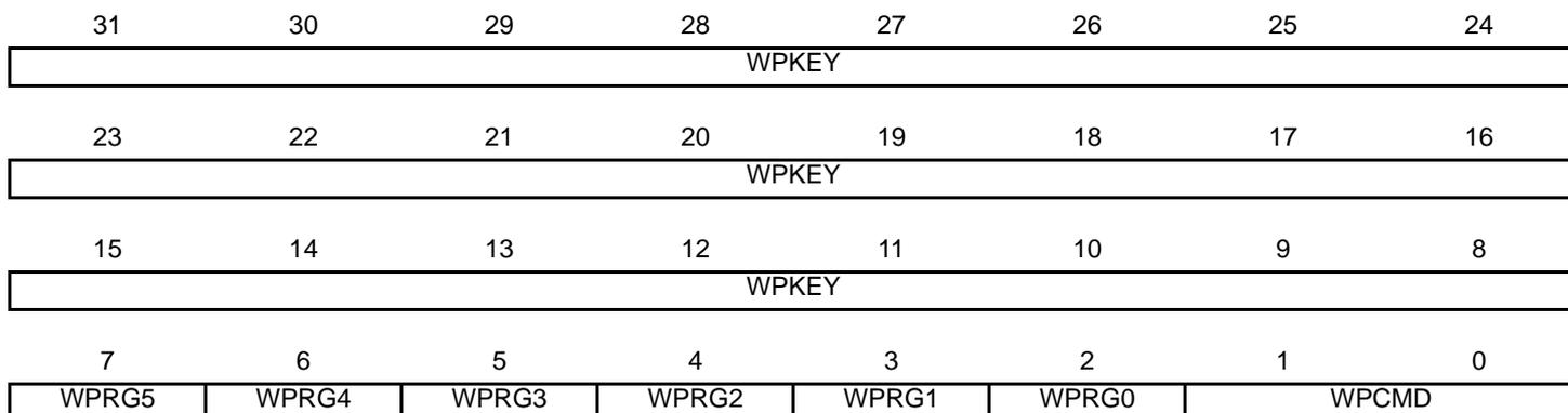
See [Section 40.6.6 “Register Write Protection”](#) for the list of registers that can be write-protected.
