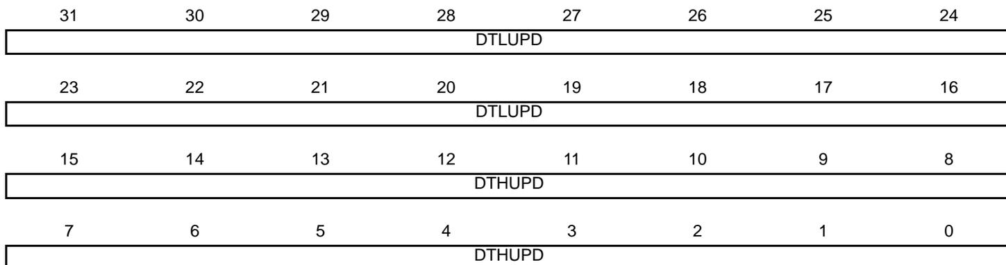
This register can only be written if bits WPSWS4 and WPHWS4 are cleared in the [PWM Write Protection Status Register](#). This register acts as a double buffer for the DTH and DTL values. This prevents an unexpected waveform when modifying the dead-time values.
