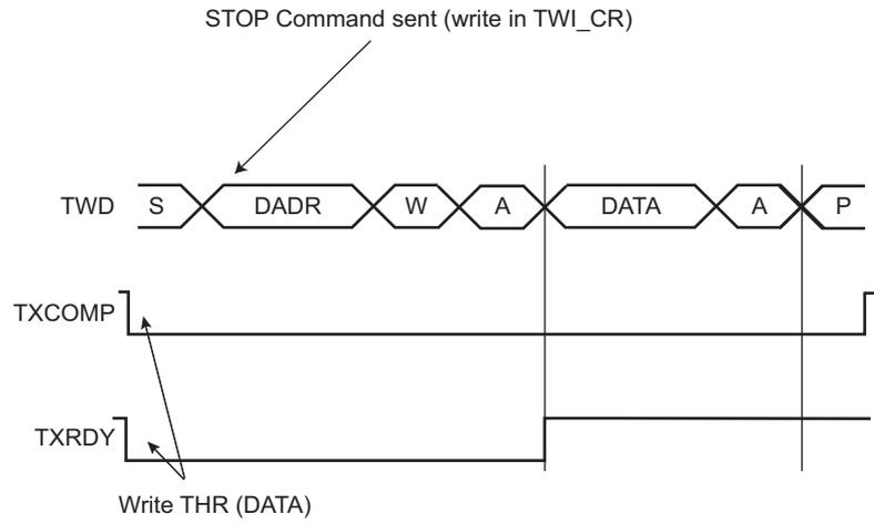
**Figure 36-7. Master Write with Multiple Data Bytes**
