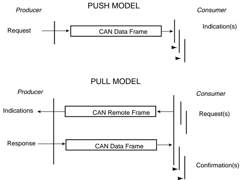
In Pull Mode, a consumer transmits a remote frame to the producer. When the producer receives a remote frame, it sends the answer accepted by one or many consumers. Using transmit and receive mailboxes, a consumer must dedicate two mailboxes, one in Transmit Mode to send remote frames, and at least one in Receive Mode to capture the producer's answer. The same structure is applicable to a producer: one reception mailbox is required to get the remote frame and one transmit mailbox to answer.
