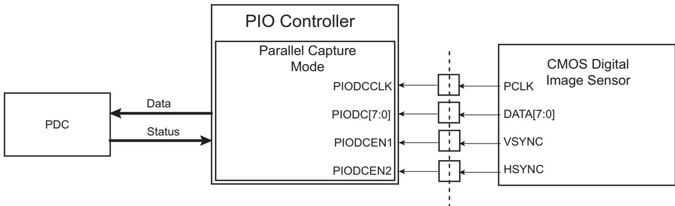
As soon as the parallel capture mode is enabled by writing a one to the PCEN bit in PIO\_PCMR, the I/O lines connected to the sensor clock (PIODCCLK), the sensor data (PIODC[7:0]) and the sensor data enable signals (PIODCEN1 and PIODCEN2) are configured automatically as inputs. To know which I/O lines are associated with
