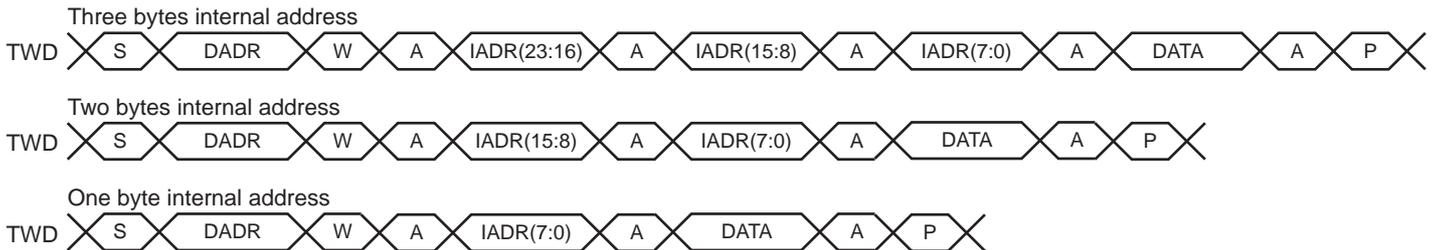
**Figure 36-13. Master Read with One, Two or Three Bytes Internal Address and One Data Byte**
