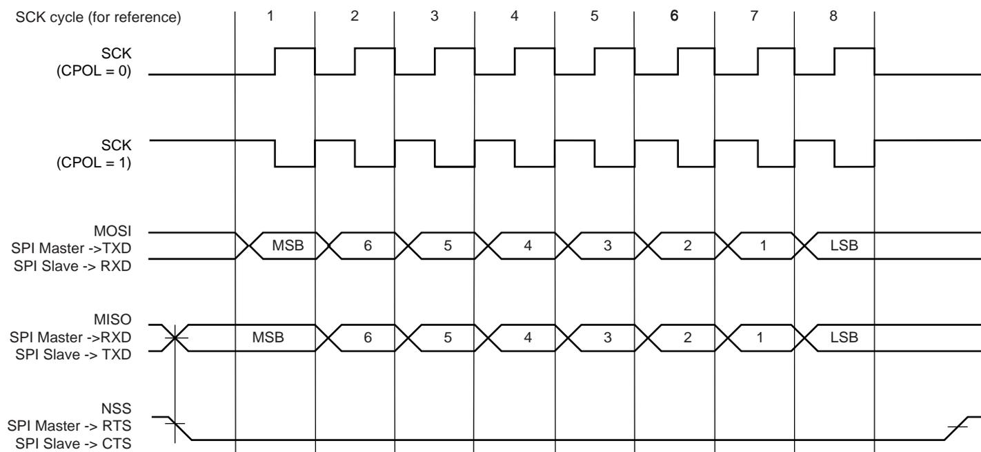
**Figure 38-39. SPI Transfer Format (CPHA = 0, 8 bits per transfer)**
