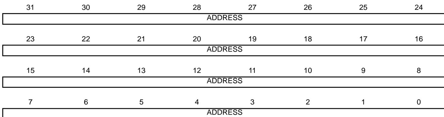
The SCB\_MMFAR contains the address of the location that generated a memory management fault.
