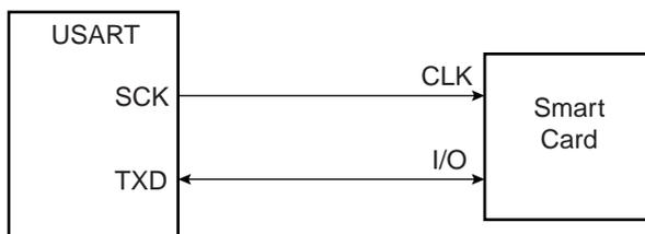
When operating in ISO7816, either in T = 0 or T = 1 modes, the character format is fixed. The configuration is 8 data bits, even parity and 1 or 2 stop bits, regardless of the values programmed in the CHRL, MODE9, PAR and CHMODE fields. MSBF can be used to transmit LSB or MSB first. Parity Bit (PAR) can be used to transmit in normal or inverse mode. Refer to “USART Mode Register” on page 927 and “PAR: Parity Type” on page 928.
