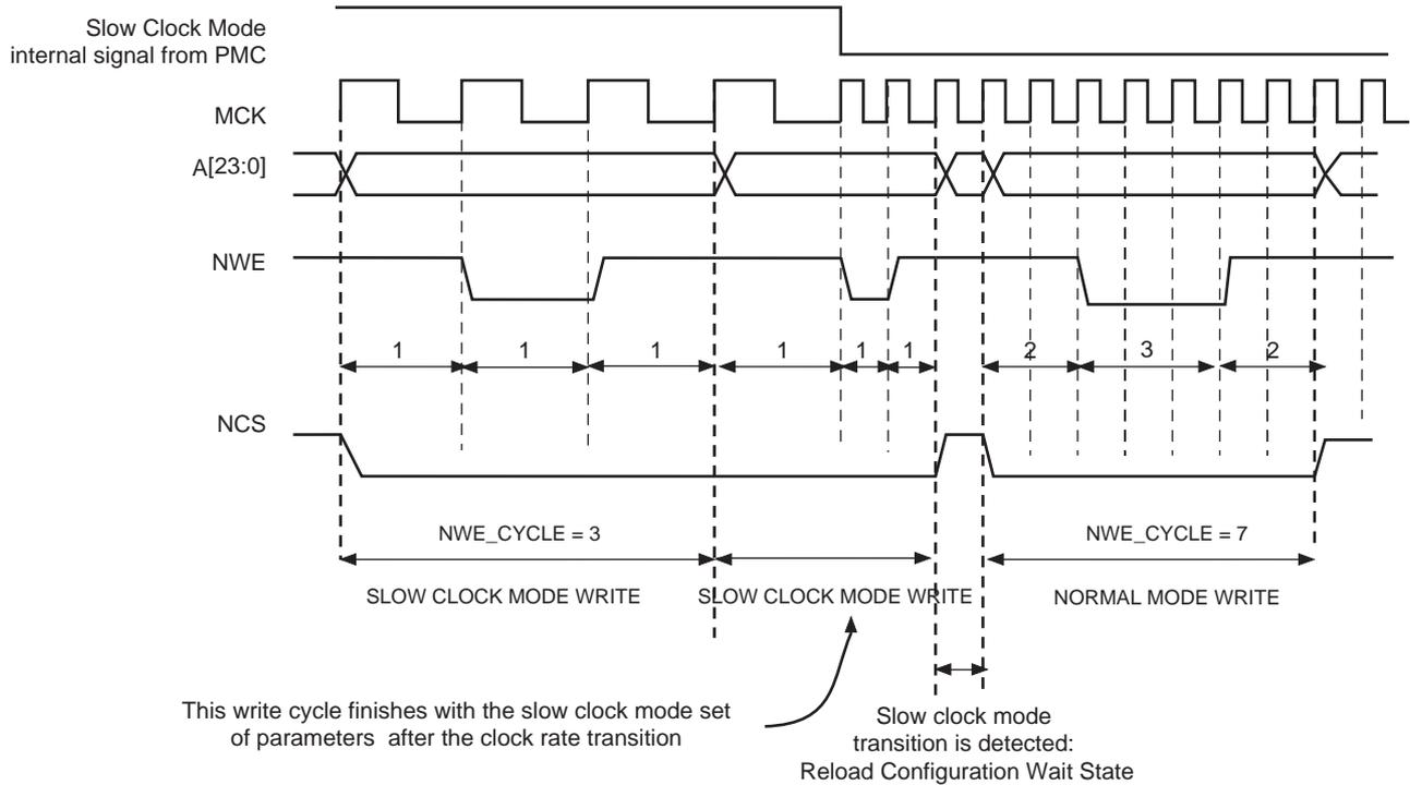
**Figure 28-30. Recommended Procedure to Switch from Slow Clock Mode to Normal Mode or from Normal Mode to Slow Clock Mode**
