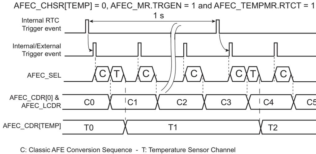
Assuming AFEC\_CHSR[0] = 1 and A\_CHSR[TEMP] = 1 where TEMP is the index of the temperature sensor channel
