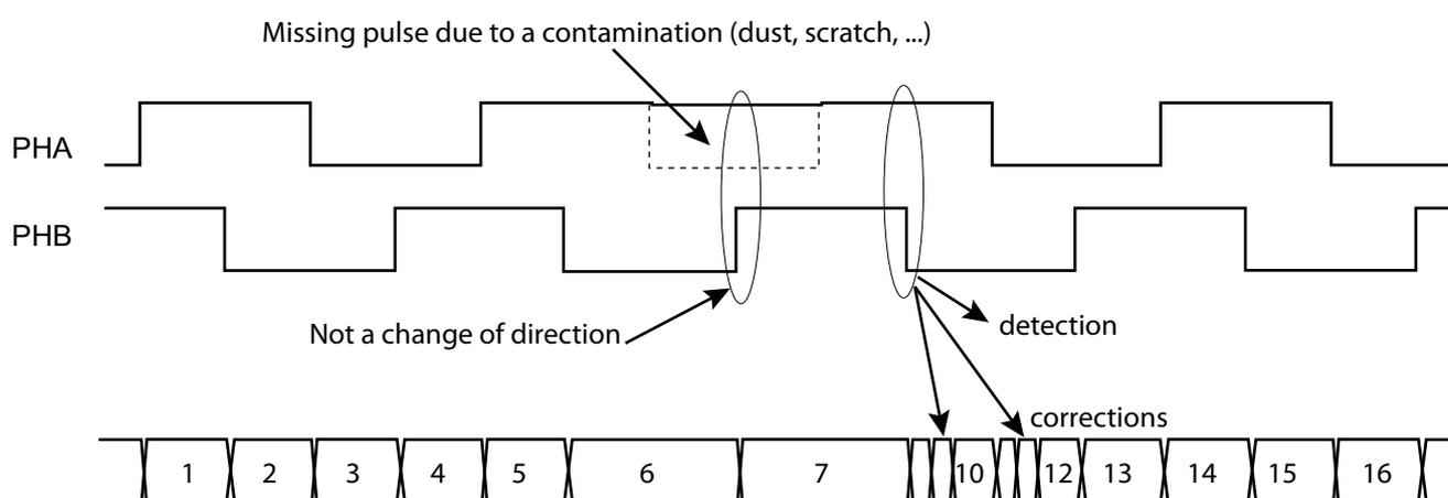
If a quadrature device is undamaged, the number of pulses counted for a predefined period of time must be the same with or without detection and auto-correction feature.
