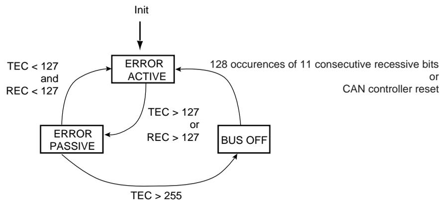
An error active unit takes part in bus communication and sends an active error frame when the CAN controller detects an error.
