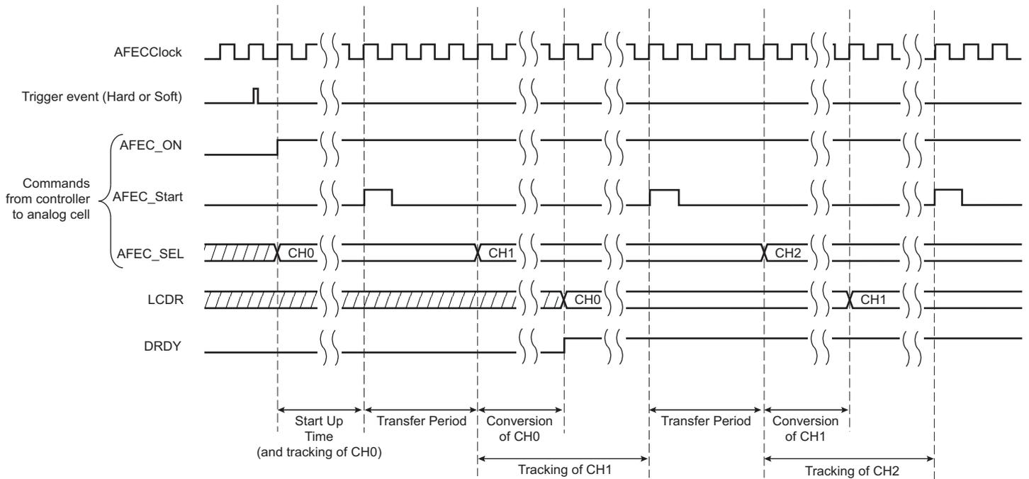
**Figure 45-3. Sequence of AFEC conversions when Tracking time < Conversion time**
