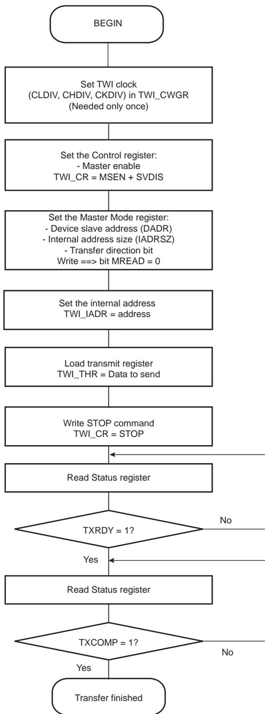
Figure 36-18. TWI Write Operation with Multiple Data Bytes with or without Internal Address
