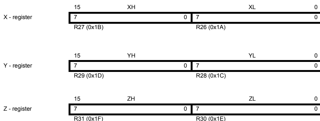
Figure 6-3. The X-, Y-, and Z-Registers
