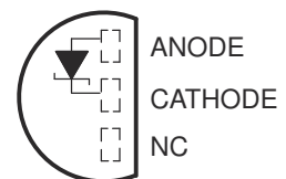
1.2 V . . . LP (TO-92/TO-226) PACKAGE (TOP VIEW)
