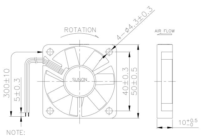
1.LEAD WIRE: UL10308 #24AWG RED WIRE----(+) BLACK WIRE----(-) 2.FRAME TYPE: RIB
